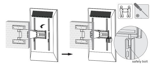
Tighten the bottom bolts to secure the display brackets to the mount.
